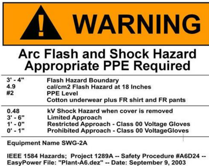
Figure 6 — Equipment Specific Field Label
